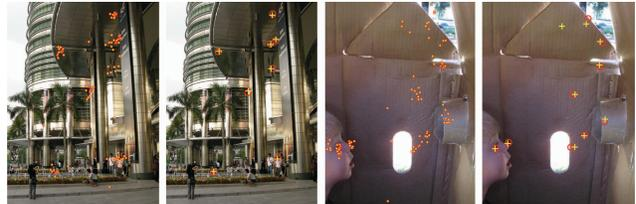
Figure 10. **Meanshift fixation detection results on two Judd images.** On left is the noisy, subsampled gaze data used for testing. On right are the detected fixations. Red circles indicate ground truth (detected in 240Hz data using code provided by Judd *et al.*) and yellow crosses indicate fixations detected in the noisy 30Hz data using our meanshift approach.
